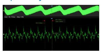
Using a hardware-based Zoom technique and record length of up to 500 Mpts, users can select a slower timebase without compromising the sample rate, and then quickly zoom in to focus on the area of interest.
