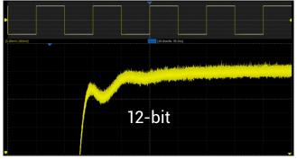
When compared to waveforms acquired and displayed using conventional 8-bit oscilloscopes, waveforms captured with 12-bit technology are cleaner and provides more signal detail. This is helpful for wide dynamic range signals in which a full-scale signal must be acquired while at the same time very small amplitude signal details must be analyzed.
