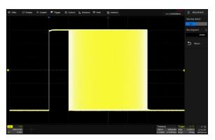
Segmented memory collection will store the waveform into multiple memory segments (up to 80,000) and each segment will store a triggered waveform as well as the dead time information. The interval between segments can be as small as 1.3 µs. All of the segments can be played back using the History function.
