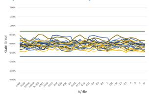
A typical DC Gain Accuracy 0.5% combined with low noise floor provides the capability to perform sensitive measurement required for wide range of applications.
