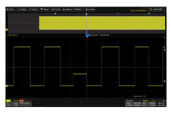
The oscilloscope can search events specified by the user in a frame. Events flagged by the Search can be recalled automatically using Navigate. It can also navigate by time (delay position) and history frames.
