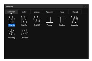
The built-in Function/Arbitrary waveform generator can output waveform with up to 25 MHz frequency and ±3 V amplitude. Six basic waveforms plus multiple types of arbitrary waveforms are built-in. (Optional 50 MHz USB AWG waveform generator module: T3DSO-FGMOD)
