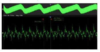
Using hardware-based Zoom technique and record length of up to 400 Mpts, users can select a slower time-base without compromising the sample rate, and then quickly zoom in to focus on the area of interest.
