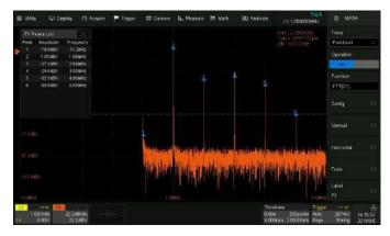
Hardware-accelerated FFT supports up to 4 Mpts operation. This provides high-frequency resolution with a fast refresh rate. The FFT function also supports a variety of window functions so that it can adapt to different spectrum measurement needs. Three modes (Normal, Average, and Max hold) can satisfy different requirements for observing the power spectrum. Auto peak detection and markers are supported.
