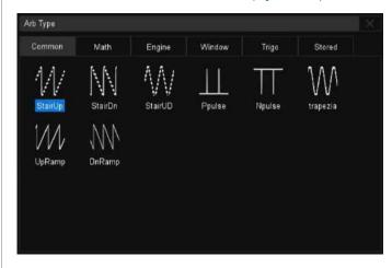
The 50 MHz waveform generator can output waveforms with up to 50 MHz frequency and ±3 V amplitude. Six basic waveforms plus multiple types of arbitrary waveforms are built-in.
