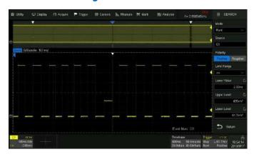
The oscilloscope can search events specified by the user in a frame. Events flagged by the Search can be recalled automatically using Navigate. It can also navigate by time (delay position) and history frames.
