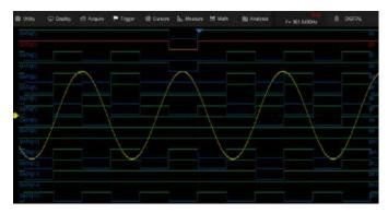
Four analog channels plus 16 digital channels enable users to acquire and trigger the waveforms then analyze the pattern, simultaneously with one instrument.
