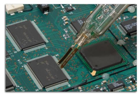
The IC leads with a compensation resistor provide excellent signal fidelity when probing pins of an IC. One side of each blade is insulated to prevent shorting the signal to the adjacent pin.
