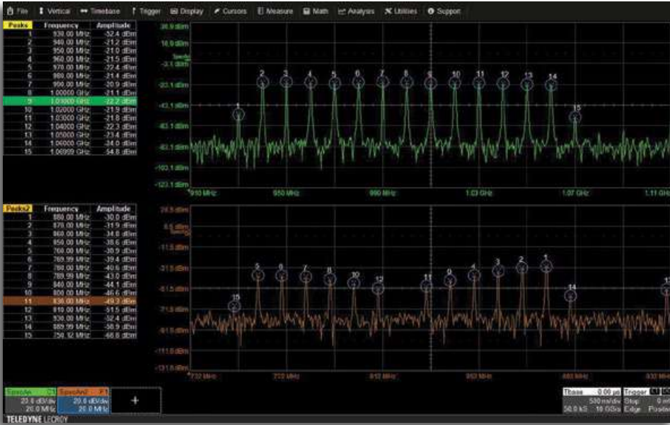
Use two independent input settings and frequency ranges for advanced spectrum analysis.
