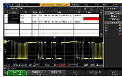
Figure 17. CAN-FD decode and trigger.
