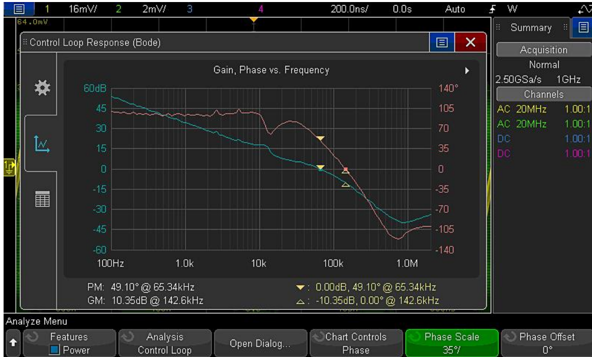
Figure 28b. New control loop response analysis (bode plot) shows the gain/phase plot over frequency sweep.
