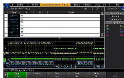
Figure 16. RS232 decode and trigger.
