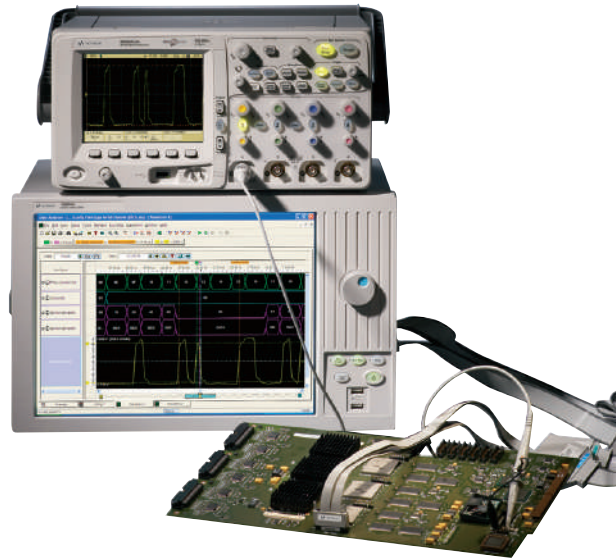
Figure 4. View Scope seamlessly integrates your scope and logic analyzer waveforms into a single display.
