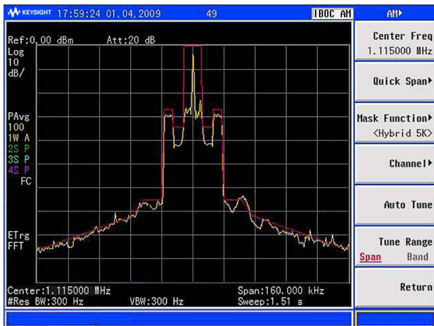
IBOC-AM measurement with N9340B IBC
